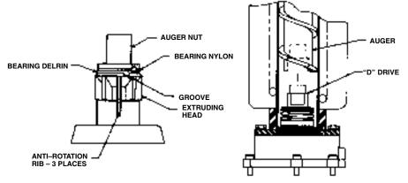
FIGURE 7. AUGER AND EXTRUDING HEAD REMOVAL
